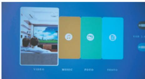
On the right side of the screen you can see the status of each of the USB ports, in blue the ports in which a pendrive is inserted and in gray the free ports. With left and right arrow keys, on the control keyboard or remote control, it is possible to highlight the box corresponding to the desired media file, then confirm with "OK" button.
