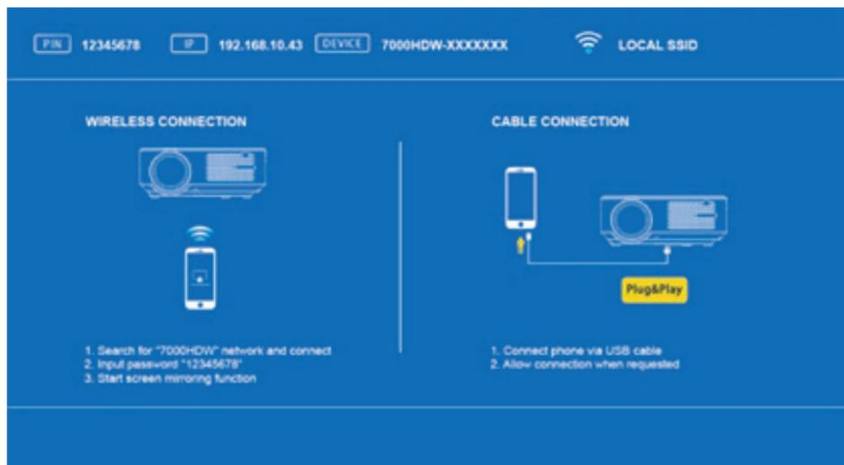
Connect the smartphone or tablet to the used wireless network and then, using the screen duplicate function, the phone screen will be reproduced by the projector. Since the image is vertically developed, rotate the device in landscape mode.
