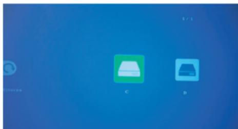
In the next screen you can view the letters corresponding to each of the two pendrives, "C" for a single pendrive inserted or "C" for USB1 and "D" for USB2 if both ports are used. With left and right arrow keys, on the control keyboard or remote control, you can select the desired pendrive, or press "Back" to go to the previous screen. Press "OK" to confirm.
