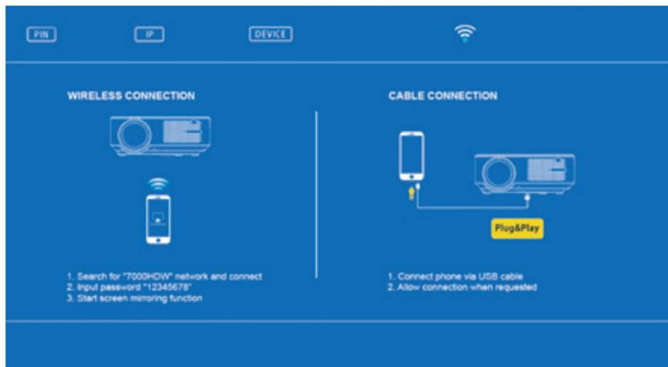
Access the smartphone or tablet menu settings and, from connections sub menu, connect to "7000HDW-XXXXXXX" using the password 12345678. The device will indicate a connection without internet access, which must be ignored.
